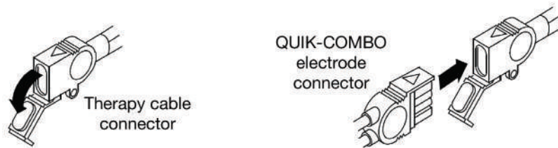
Figure 36 Connect QUIK-COMBO Electrodes to Therapy Cable
